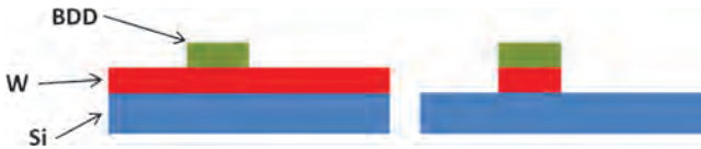
Figure 16.14 Schematic of the two different circuits assessed for shunted SQUIDs. The blue layer is the silicon wafer, the red layer is tungsten (20 nm and 50 nm) and the green layer is boron-doped diamond (BDD).
