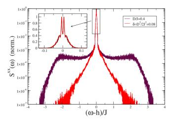
FIG. 2. (Color online) ESR line shape (high-energy tail) for a one-dimensional chain  $(T \gg J)$  for the Dzyaloshinskii-Moriya and XXZ models (using  $2\delta = D^2/J^2$ ). The response is identical only at low energy (inset).
