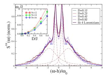
FIG. 1. (Color online) ESR line shape of a one-dimensional chain of N=16 spins  $(T\gg J)$ . The curves are rescaled with the half width at half maximum,  $\omega_0/J$  (shown in the inset as a function of D/J for three sizes).
