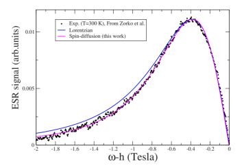
FIG. 10. (Color online) ESR signal (derivative of the resonance line at  $\omega < h$ ): theory and experiment on the kagome  $S = \frac{1}{2}$  ZnCu<sub>3</sub>(OH<sub>3</sub>)Cl<sub>2</sub> (from Ref. 32).
