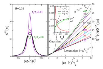
FIG. 6. (Color online) ESR line shape for infinite onedimensional chains, assuming different cutoffs  $\tau_0$  of the diffusive tail. The arrow (inset) indicates the self-consistent  $\tau_c$ .
