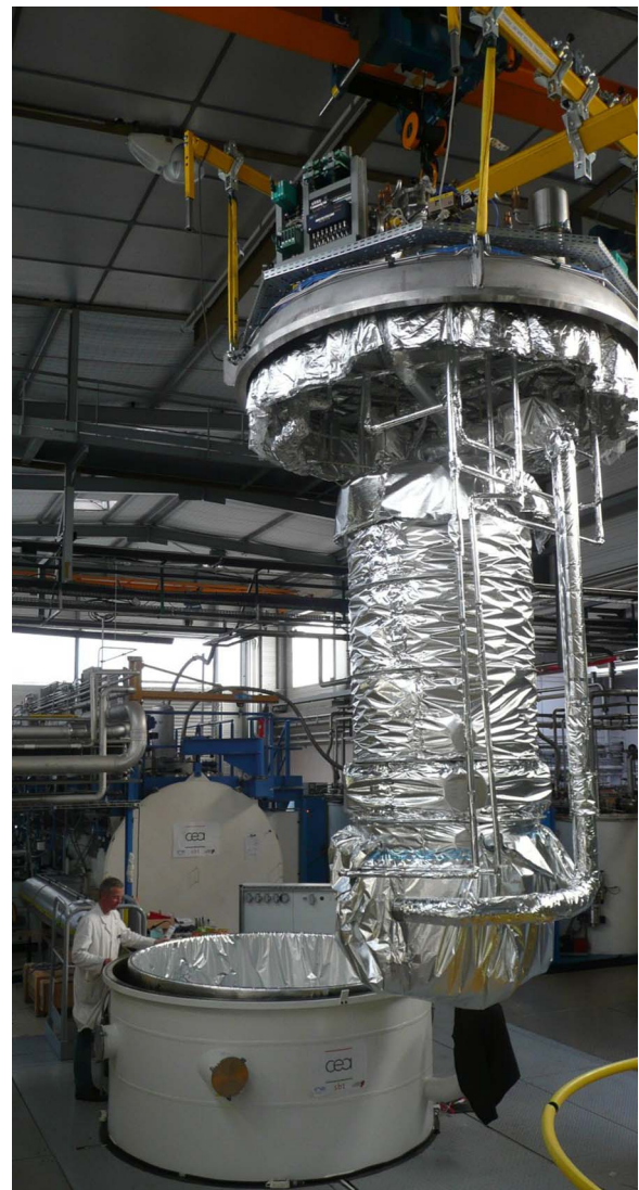
FIG. 8. Insertion of the saturated bath (covered with MLI) into the Multipurpose cryostat.
