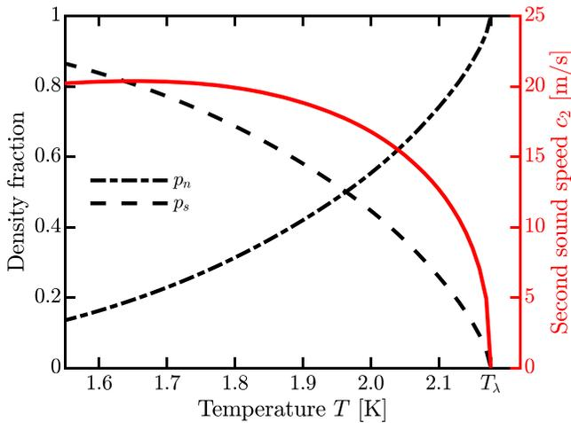
**FIG. 1.** Left axis: temperature dependence of the density fractions of the normal ( $p_n$ , dot-dashed line) and superfluid ( $p_s$ , dashed line) components of He II. Right axis: temperature dependence of the second sound speed (solid line).  $T_\lambda \approx 2.2$  K denotes the superfluid transition at the saturated vapor pressure. Data from Ref. 7.
