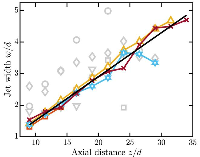
**FIG. 10.** Peak width  $w$  as a function of the axial distance  $z$  (both quantities are normalized by the nozzle diameter  $d$ ). Color symbols: points with  $L_0 > L_t$ , i.e., datasets A2 (in part), A3, B3, and B4, collectively named high set; gray symbols: remaining points, with  $L_0 \leq L_t$ , i.e., datasets A1, A2 (in part), B1, and B2, collectively named low set. Note that the symbols are as in Fig. 9, regardless of their color; black line: linear fit, Eq. (10).
