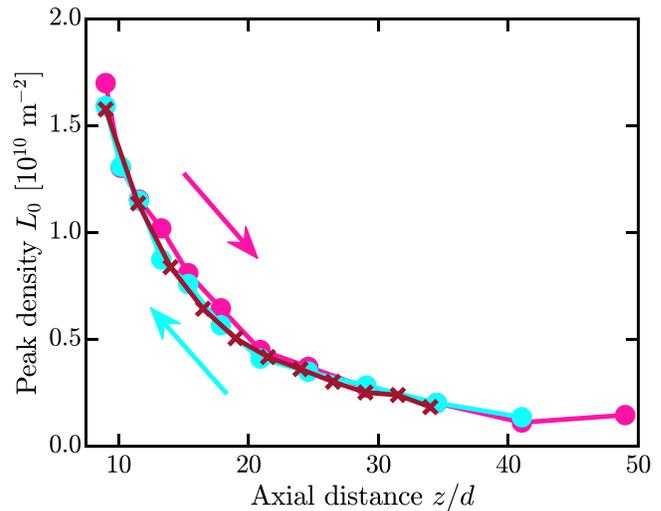
FIG. 8. Peak vortex line density (i.e., density along the jet axis)  $L_0$  as a function of the axial distance  $z$ , normalized by the nozzle diameter  $d$ , for datasets B4 (red crosses) and C1 (cyan and magenta points). Color arrows denote the direction of the sensor stroke (receding from or approaching toward the nozzle).
