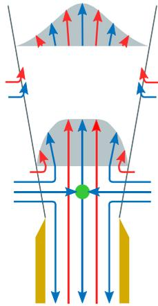
**FIG. 2.** Sketch of the two-component flow field in a thermal counterflow jet. Red (blue) arrows: normal (superfluid) component; green point: stagnation point of the superfluid component. Displayed are also velocity profiles in the near field, i.e., in the close proximity of the nozzle (bottom) and in the intermediate field (top), see Eq. (4). Adapted from Ref. 22.
