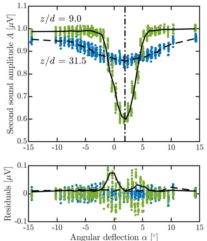
FIG. 4. Top panel: two sets of 30 sweeps (points) across the jet axis, obtained at 1.65 K and 776 mW (dataset A3) for  $z/d = 9.0$  and  $31.5$ , as indicated in the figure. Solid and dashed black lines: ensemble-averaged data used for the calculation of the quantized vortices’ density. Dot-dashed black line: deflection offset  $\alpha_0 \approx 1.9^\circ$ , Eq. (7). Bottom panel: residuals (points) and standard deviations (lines) corresponding to the data displayed in the top panel.
