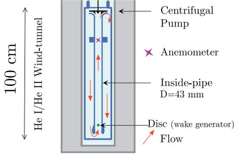
Fig. 1: (Color online) Wind tunnel (in blue) in the cryostat (in gray).
