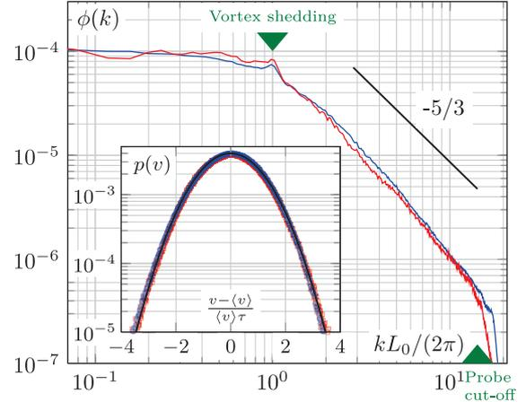
Fig. 2: (Color online) Experimental 1D velocity power spectrum above and below the superfluid transition. Red line:  $T = 2.2$  K  $> T_\lambda$  at  $R_\lambda \approx 1640$ . Blue line:  $T = 1.56$  K  $< T_\lambda$ . Inset: velocity probability density distribution above and below the superfluid transition. Black line: Gaussian distribution.
