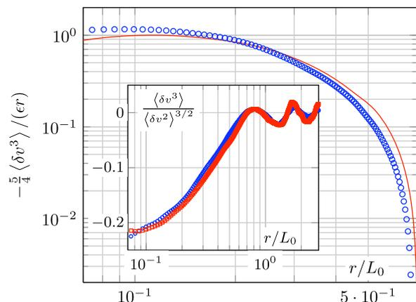
Fig. 4: (Color online) Experimental third-order velocity structure function compensated by the 4/5-law (eq. (9)) obtained in superfluid helium at  $T = 1.56$  K (blue circles) and in classical liquid helium at  $T = 2.2$  K (red squares). Inset: skewness of the distribution of longitudinal velocity increments (same color code). The smallest abscissa  $r/L_0 = 7 \times 10^{-2}$  corresponds to the probe cut-off. The oscillation at large scales is related to the frequency of the vortex shedding.
