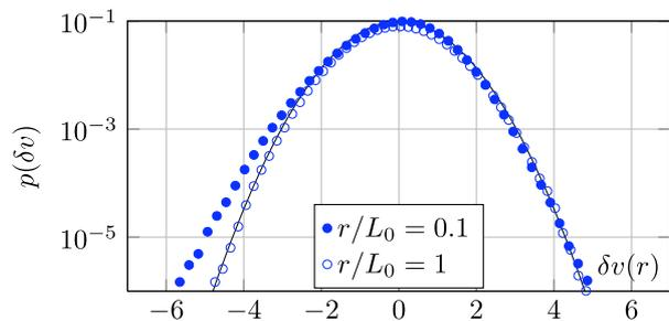
Fig. 3: (Color online) Experimental histogram of the longitudinal velocity increments at large and intermediate scales in a superfluid turbulent flow ( $T = 1.56$  K). Solid black line: Gaussian PDF.
