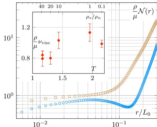
Fig. 7: (Color online) Compensated effective viscosity *vs.* scale obtained in numerical simulations at high temperature (chocolate squares) and very low temperature (sky blue circles) for nearly the same Reynolds number. Inset: effective viscosity estimated from the “plateau” of  $\mathcal{N}(r)$  for various temperatures.
