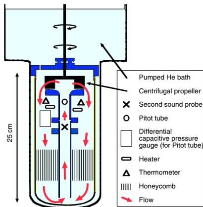
Fig. 1: Scheme of the flow loop with probes.
