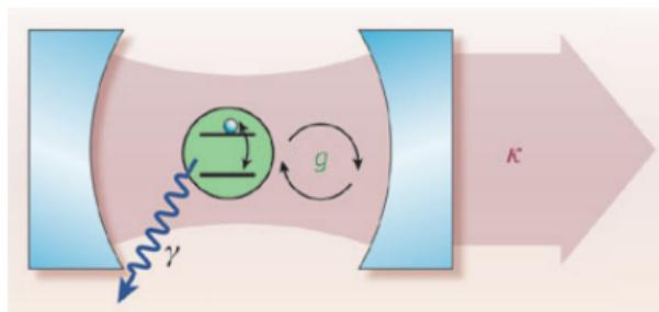
Rabi model :  $H = \omega_0 a^\dagger a + \Delta \sigma_x + g(a^\dagger + a)\sigma_z + H_{\text{out}}$
