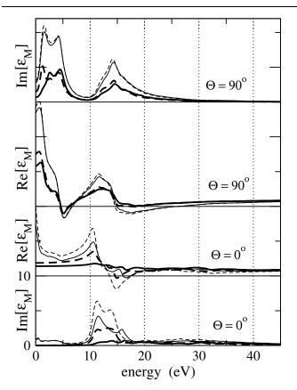
FIG. 2. Calculated  $\text{Im}[\varepsilon_M]$  and  $\text{Re}[\varepsilon_M]$  for two different **q** polarizations (in-plane  $\Theta = 90^\circ$  and perpendicular-to-plane  $\Theta = 0^\circ$ ). Dashed lines are obtained without, continuous lines including LFE. A broadening of 0.5 eV was used. The thick lines denote the results with the double interlayer spacing.
