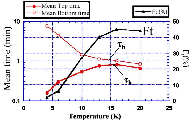
Fig.5: Temperature evolution of the top and bottom time and mean b occupation time  $F_t = \tau_h / (\tau_h + \tau_b)$ . This is consistent with temperature activated mechanism.
