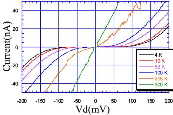
Fig.1:  $I_D$ - $V_D$  curve of a  $2\mu\text{m} \times 40\text{nm} \times 15\text{nm}$  SOI wire when varying temperature. A strong non linearity is visible at low temperature.
