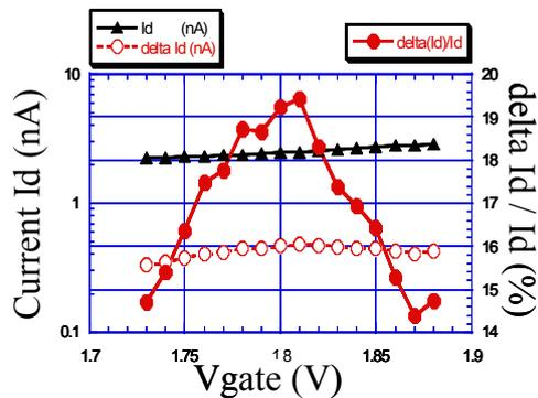
Fig.6: Gate voltage dependence of the current amplitude modulation. Note the non monotonous behaviour and the absolute level. In some cases up to 40% modulations were measured.
