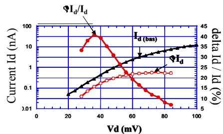
Fig.7 : Source-Drain voltage dependence of the current  $I_d$ , absolute  $\Delta I_d$  and normalised  $\Delta I_d / I_d$  current modulation.
