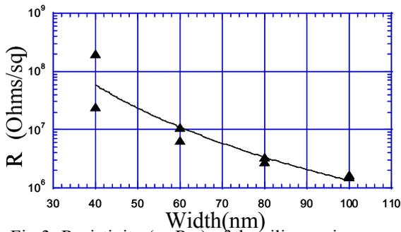
Fig 3: Resistivity ( $\rho=R.e$ ) of the silicon wires versus the wire width.  $\rho$  is not constant. This could be attributed to a reduction of the effective conducting section (surface roughness) or could either be the signature of a microscopic more complex conduction law.
