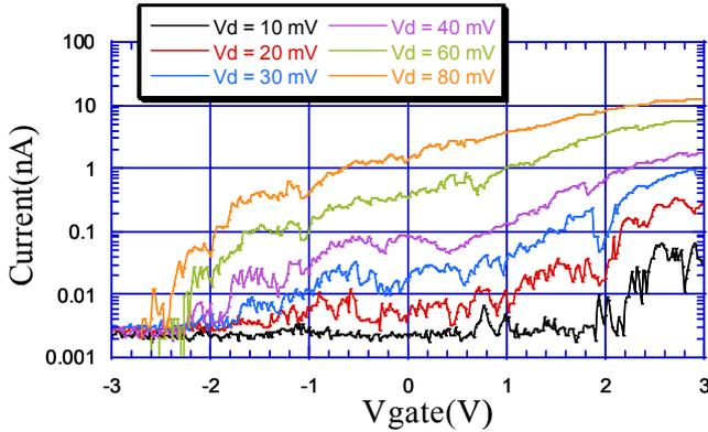
Fig 2: Gate voltage dependence of the  $I_{SD}$  current for various  $V_{SD}$  bias. Each curve is complex yet totally reproducible.
