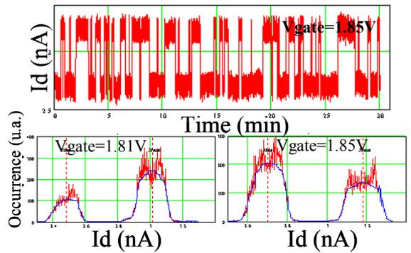
Fig.4: Time evolution of the  $I_{SD}$  current in stationary bias conditions. The evolution of the amplitude occurring for two different Gate bias is clearly visible on the histogram of the amplitude.
