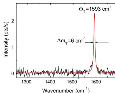
Fig. 3. Raman signal corresponding to the tangential modes of SWNTs deposited on thermally oxidized Si substrate and its Lorentz fit into three peaks at  $1599 \text{ cm}^{-1}$ ,  $1590 \text{ cm}^{-1}$ ,  $1581 \text{ cm}^{-1}$  with  $5\text{--}7 \text{ cm}^{-1}$  width at half maximum.
