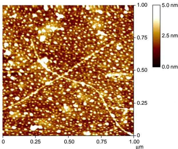
Fig. 2. AFM topography of SWNTs grown on a thermally oxidized Si substrate which puts forward two crossing nanotubes surrounded by catalytic particles.
