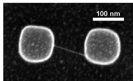
Fig. 5. SEM images of suspended SWNTs (in the limit of an isolated SWNT) self assembled by HFCVD between thermally oxidized Si pillars with a 200-nm interdistance and capped with a 2-nm thick Co layer.
