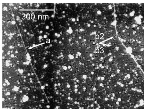
Fig. 1. SEM image of SWNTs grown on a thermally oxidized Si substrate with a 2-nm thick cobalt layer. Arrows underline the position of the SWNTs: a straight one (a) and a small bundle ( $b_1$ ) which splits off into two thinner ones ( $b_2$ ,  $b_3$ ).
