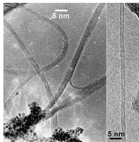
Fig. 4. TEM observations of an isolated SWNT and small SWNT bundles synthesized on Mo grids covered with a 2-nm thick Co layer.
