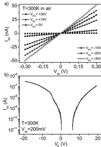
**Figure 1.** (a) Drain–source  $I$ – $V$  characteristics of a standard unipolar p-type device (wafer A) at 300 K in air for different back-gate voltages. (b) Transfer characteristics at 300 K in vacuum for a typical back-gated ambipolar device (wafer A).
