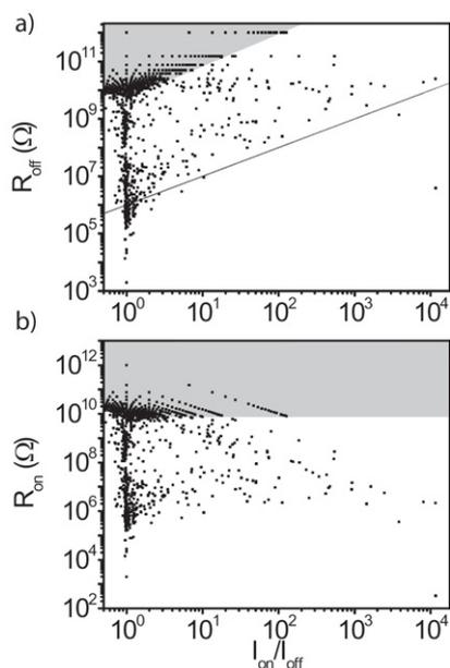
**Figure 5.** (a) Resistance in the *off* state for wafer B plotted versus the *on-to-off* current ratio. The line corresponds to the calculated  $R_{\text{off}}$  with our model. (b) The same for resistance in the *on* state. In both cases, the grey zones correspond to the detection limit of the set-up.
