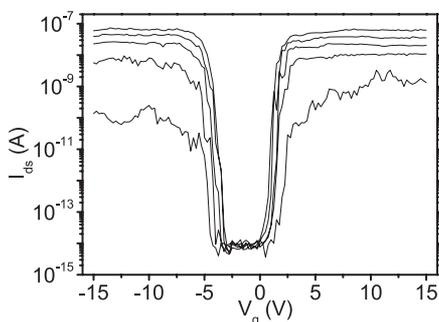
**Figure 9.** Top gate transfer characteristics of a CNFET using a 100 nm thick Parylene layer as the top gate dielectric. The measurement was performed at  $T = 6 \text{ K}$ , with both top and back gates polarized with gate sweep rate of  $-100 \text{ mV s}^{-1}$ . The drain–source voltage is increased by 100 from 100 to 500 mV from bottom to top.
