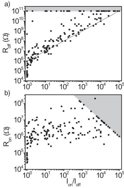
**Figure 3.** (a) Resistance in the off state plotted versus the on-to-off current ratio for wafer A. The line corresponds to the calculated  $R_{\text{off}}$  with our model. (b) The same for resistance in the on state. In both cases, the grey zone corresponds to the detection limit of the set-up.
