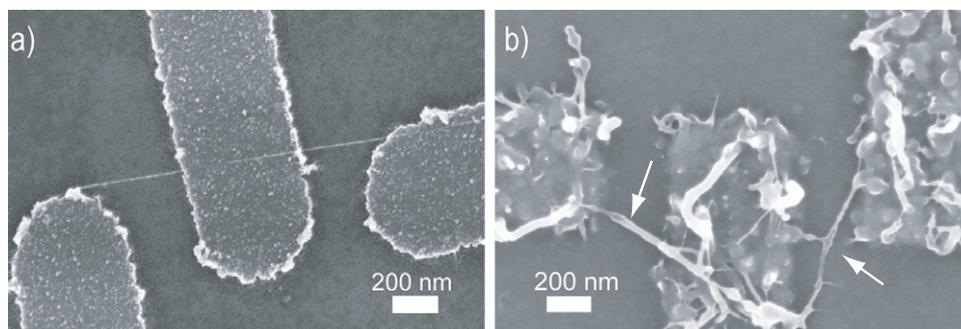
**Figure 6.** SEM micrographs showing (a) an as grown CNFET and (b) a typical CNFET after deposition of a 20 nm thick Parylene C layer. A conformal coating recovers the nanotube channels (arrows).
