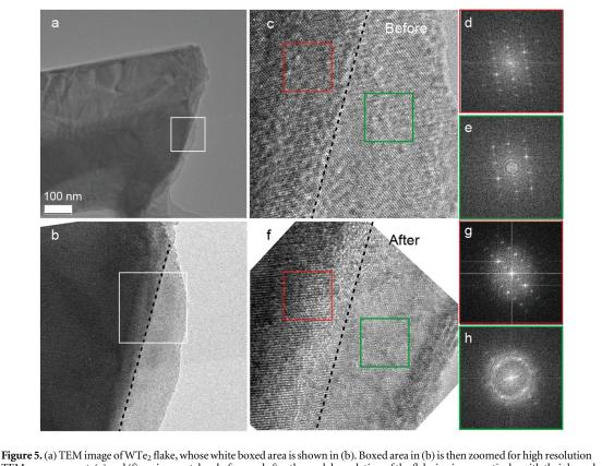
TEM measurement. (c) and (f) are images taken before and after thermal degradation of the flake in air, respectively, with their boxed area performed FFT, as shown in (d)–(e) and (g)–(h). Dashed lines in (b)–(f) highlights the boundary between thick and thin WTe<sub>2</sub>. Notice (f) is rotated to align with (b) and (c) for visual clarity.
